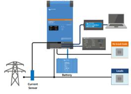
Standard mobile or off-grid application with external current sensor Maximum current sensing range: 50A resp 100A
